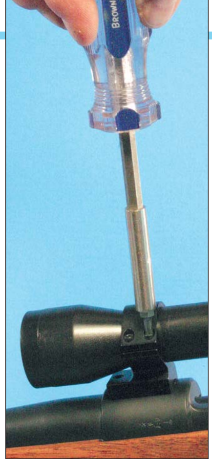
Scope tubes are of relatively thin aluminum. If ring screws are turned too tightly, the rifle might start grouping as if the action screws are actually loose.
