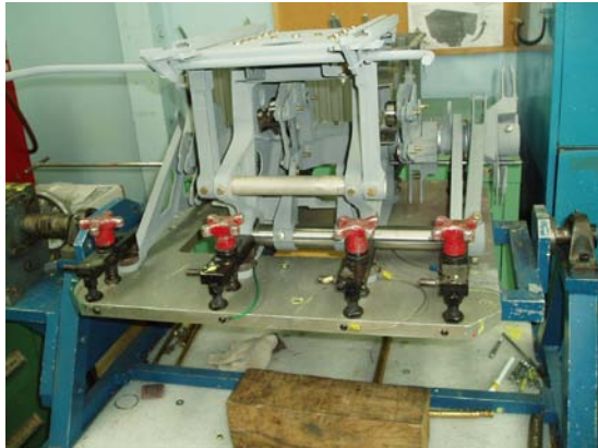
Figure 3.1 UH-60 Flight Controls Mixer Figure 3. 2 S haft Part no. 70400-02155-103
