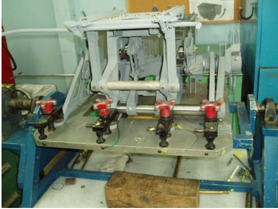
Photo 1. UH-60 Flight Controls Mixer Assembly
